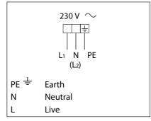
Figure 16b Connecting the feeder cable
